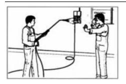
High pressure water jets can be dangerous. Do not direct the water at any person, animals or electrical equipment, or towards the machine.
