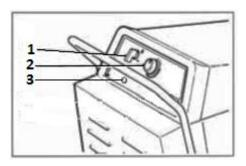
Turn ON the main switch (1) Adjust the temperature required by the thermostat (2)
