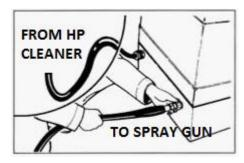
Connect the high pressure hose from the High Pressure Cleaner to the inlet of the Hot Box.
