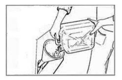
Check the level of the fuel and fill with clean diesel if required.
