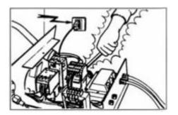
Always disconnect the plug before commencing any servicing work on the machine (do the same during installation).
