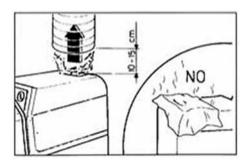
Do not use the burner in buildings or confined spaces without adequate ventilation. Do not touch or cover the exhaust.
