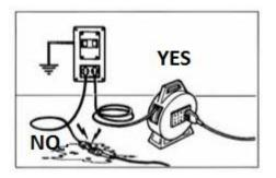
Be sure your electric plug complies with the safety rules in force. The plug must be properly and securely connected with an approved earth terminal. If you want to use an extension cable always use a cable reel with proper section cable.
